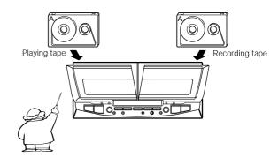
• When recording is started, the tape will be transported in the direction selected in this step.
